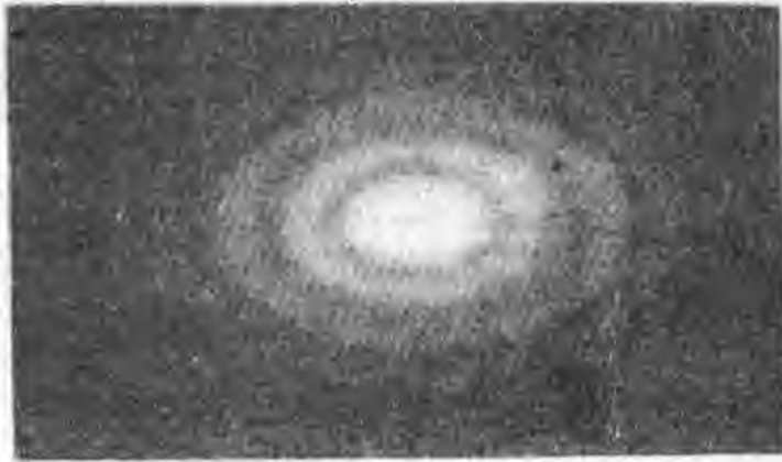
Fig. 3.7 The diffraction of light. Light brought to a focus does not come to a point, but gives rise to a blurred disc of light surrounded by several dark and light bands (the 'Airy disc'). (W. H. A. Pincham.)
